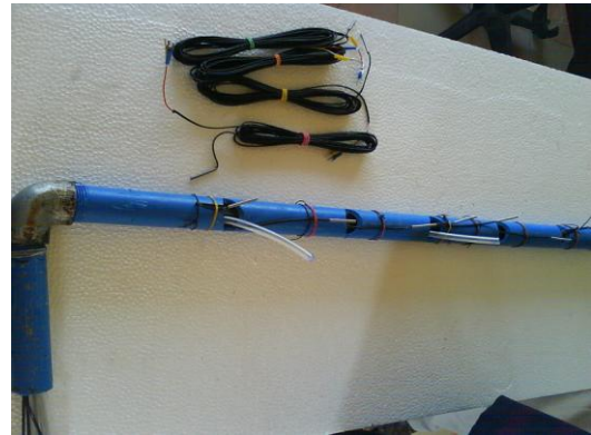
Fig. 2. Arrangement of K-type thermocouples to measure the temperature of various zones of solar-pond.
